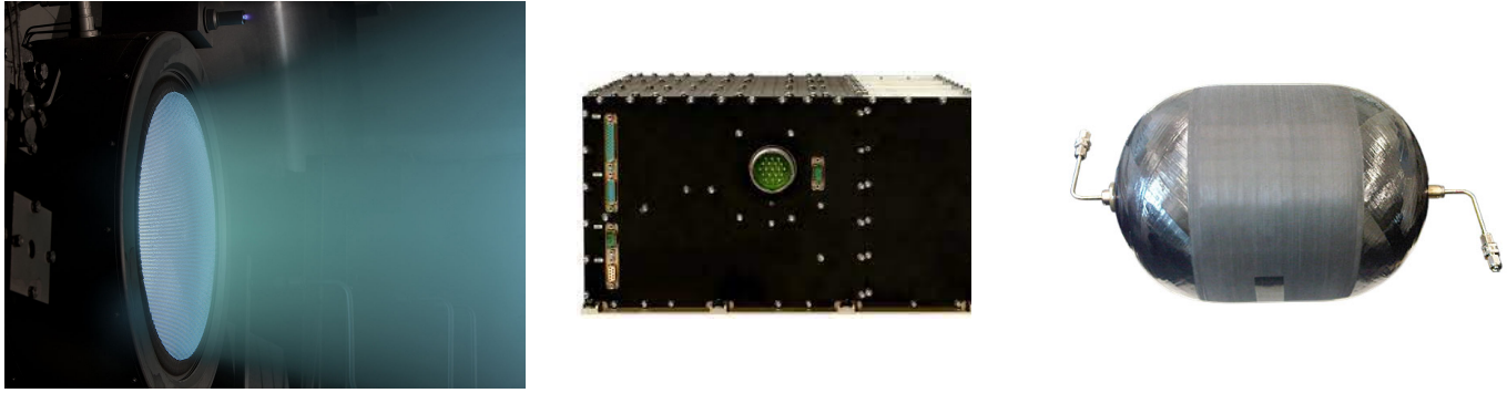
Figure 7.3.7: NEXT 9a Ion Thruster (left), PPU (middle), & Xe Propellant Tank (right)
