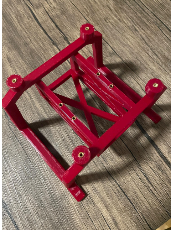
Figure 8: First Drone Legs Prototype with Heat Set Inserts
